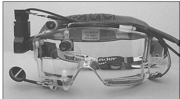
Figure 1 Custom-built headgear for the wearable eye tracker.
