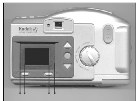
Figure 7 The camera's LCD preview panel was masked to limit the field-of-view during image capture.
