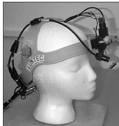
Figure 5 Close-up of headgear with head-position sensor.
