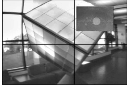
Figure 3 Video image of the scene with the eye image superimposed in the upper right corner. The crosshairs indicate point of gaze.
