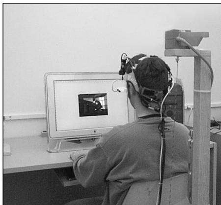
Figure 4 Magnetic transmitting and eye tracking setup.
