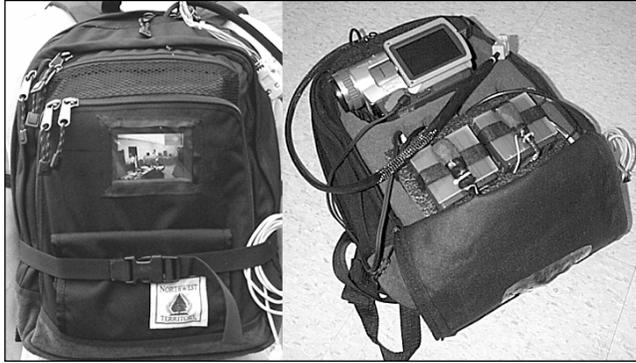
Figure 2 Wearable eye tracking backpack containing a digital video camcorder, picture-in-picture, ASL control unit, and batteries. The LCD is visible through the backpack to facilitate setup.
